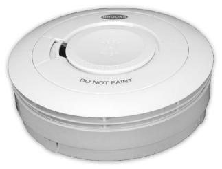
The EIB650IWX is an externally powered Photoelectric Smoke Alarm, designed to be used with the Brooks range of Residential Fire Panels, when installed in conjunction with a compatible interface base. They are particularly responsive to smouldering fires and the dense smoke given off by such things as foam filled furnishings or overheated PVC.
